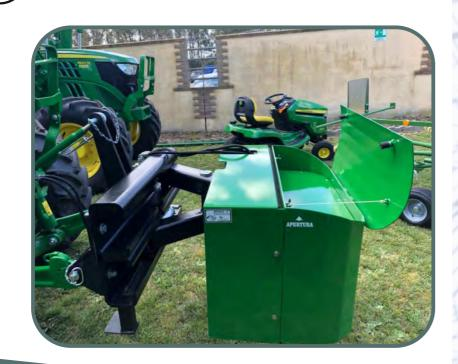
The operator can hydraulically balance the tractor's weight between the rear and front wheels by extending the counterweight away from the tractor's nose by up to one metre, depending on requirements. The following is a list of its advantages:
